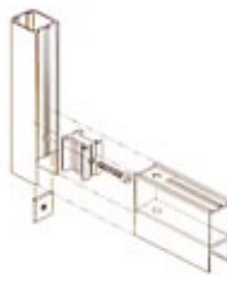
INTERNALLY BOLTED AND SCREWED OR FOUR POINT WELDED
